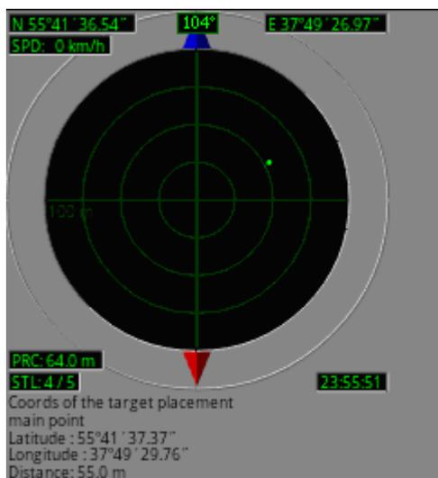
Radar provides a graphical display of the destination point relative to current movement directions. Radar indicates the direction to the geographic North Pole (acts as a Compass), and also reflects current coordinates and status of the device.
