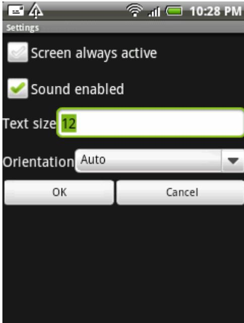
If an option «Screen always active» is selected, it will not allow an operating system to turn the screen off and put a mobile device in a standby mode.
